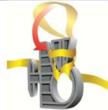
**STEP 4:** Twist the tendon to form a loop. Fold the tendon loop back down over the post.
