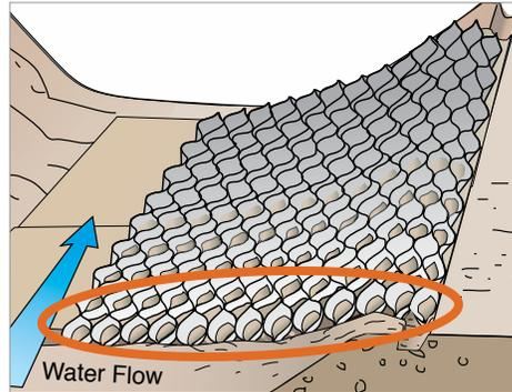
**6** Connect GEOWEB® sections with ATRA® keys. Connect side to side (A) and end to end (B).
