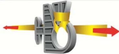
**STEP 5:** Pull the tendon so the slack is eliminated and it is tightly secured to the clip.
