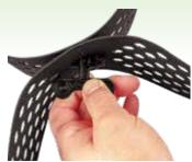
ATRA Keys, made from weather-resistant polyethylene, are 3 times stronger and 3 times faster than stapling. ATRA Keys are inserted through adjoining GEOWEB cell walls, turned and locked for the most secure and fastest connection.
