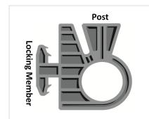
**Figure 1.** ATRA® Tendon Clip Load Transfer Device.
