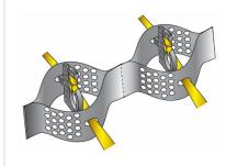
Figure 3. ATRA® Tendon Clip Locked through the GEOWEB Cell I-Slot and Properly Wrapped Tendon to Complete the Load Transfer.
