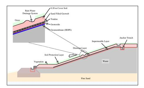
New covering system using the sand-infilled Geoweb system.
