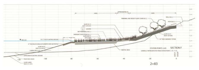
*Figure 1.* Cross section of shoreline. With the dual goal of repairing and beautifying the lake system, the designer developed a range of shoreline treatments: geotextiles for soil separation, geocellular reinforcement.
