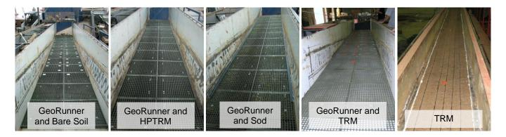
The sod and TRMs were secured on top of soil embankments using 6-inch 10-gauge turf staples; and the GeoRunner<sup>®</sup> Flow Protection Mats were secured on top of the sod and TRMs using soil anchors per the manufacturer's recommendations. Prior to hydraulic testing, bed-elevation profiles were measured in 2-ft intervals along the left side, centerline, and right side of the flume.
