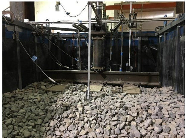
(b) Track loading test
