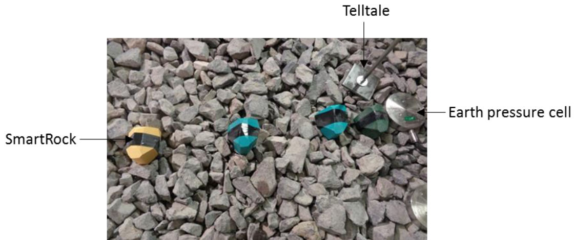
Figure 3. Earth Pressure Cells, Telltales, and SmartRocks
