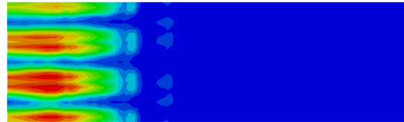
Subgrade pressure concentrations without GEOWEB geocell.
