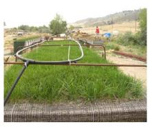
The turf reinforcement mat was secured over the textured/perforated Geoweb section by ground staples at defined intervals in conformance with the manufacturer's recommendations. The integrated system was positioned in a planter test box at a 2H:1V slope angle. Vegetation was established over a 14 week period to allow root system integration within the perforated cells of the Geoweb material. Kentucky bluegrass was the chosen vegetation for this series of tests.
